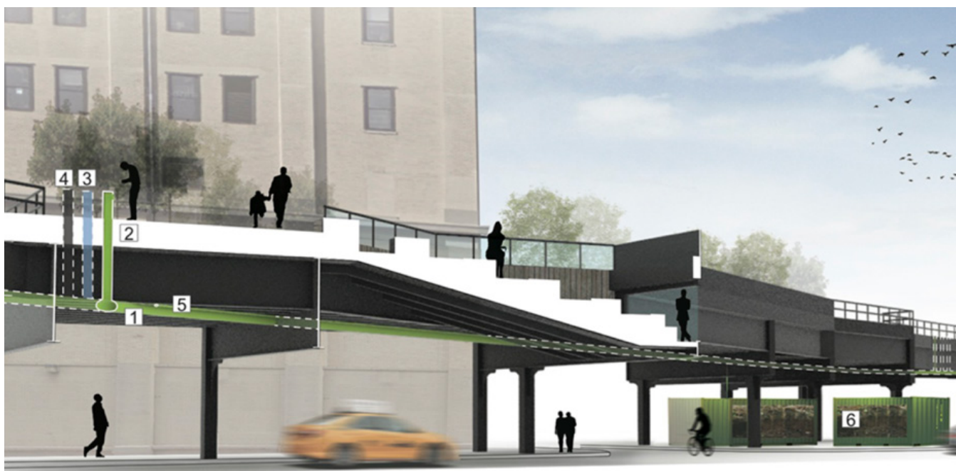
1 Pneumatic Tube; 2 Inlet for Food Waste; 3 Inlet for Recycling; 4 Inlet for Refuse; 5 Pneumatic Tube for Restaurant Food Waste; 6 Micro Anaerobic Digester
